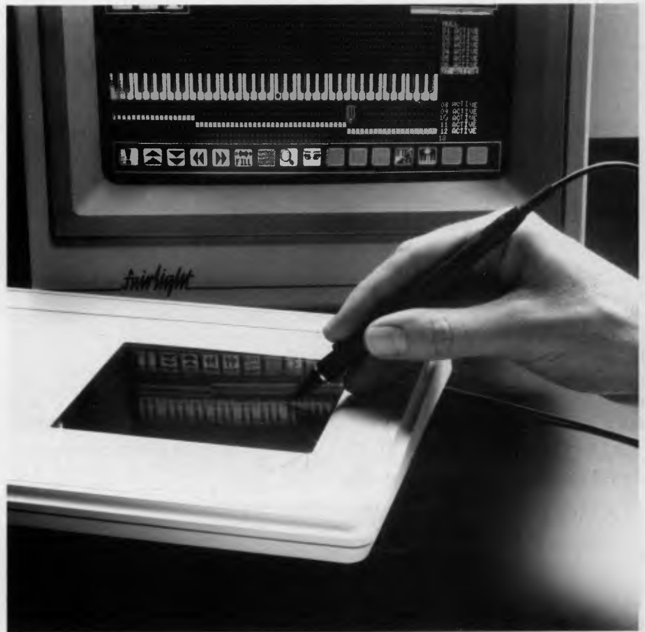
Figure 1. Fairlight's CMI (Computer Musical Instrument) Series III incorporates twelve microprocessors for each group of sixteen voices: a dual-6809 CPU (and 1 Megabyte of system RAM), which is used primarily for graphics and disk control, plus two Motorola 68000s and eight 6809 peripheral processors.
