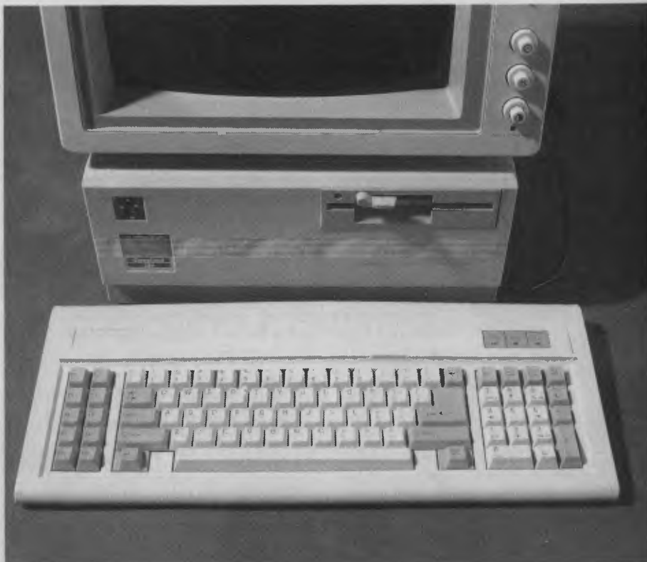
Figure 1. The 84-key layout is standard, with Caps Lock, Num Lock and Scroll Lock indicators in the upper right corner. Even though the cable plugs into the centre back of the computer, it's long enough to set the computer on the floor and the keyboard on the desk.
