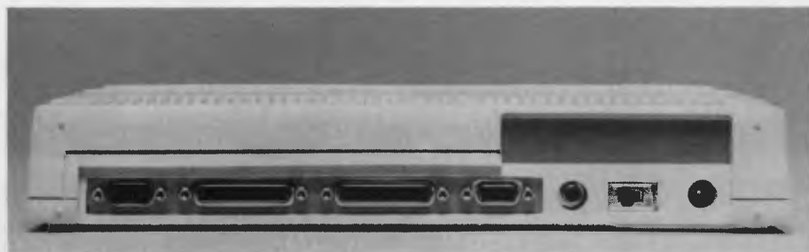
Figure 2. The back of the T1000 has a mouse, parallel printer, serial, colour monitor and composite monitor ports, a mains socket and a power switch. And, there's a plate behind which you can install the optional (Australian made) modem card.
