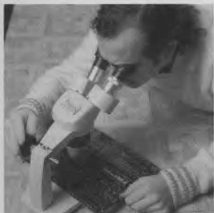
Checking the workmanship on a circuit board manufactured at Cleveland's Hendra, Queensland, plant.
