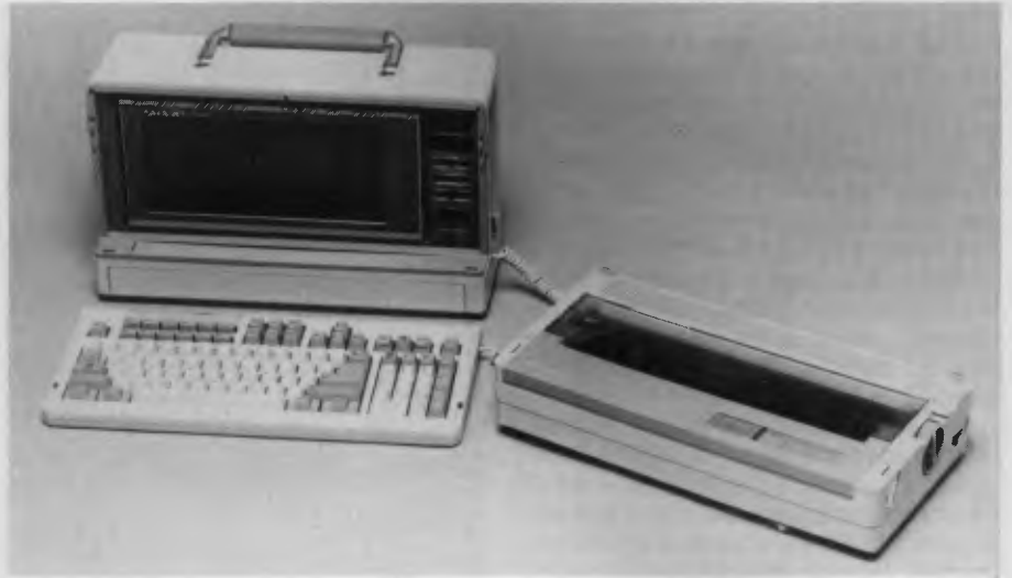
Figure 7. The Sharp printer offers Very Near Letter Quality, at a rated 20 characters per second, 10 characters to an inch, Near Letter Quality at 40 characters per second, and Draft with 72 characters a second. An optional font card gives it additional fonts.
