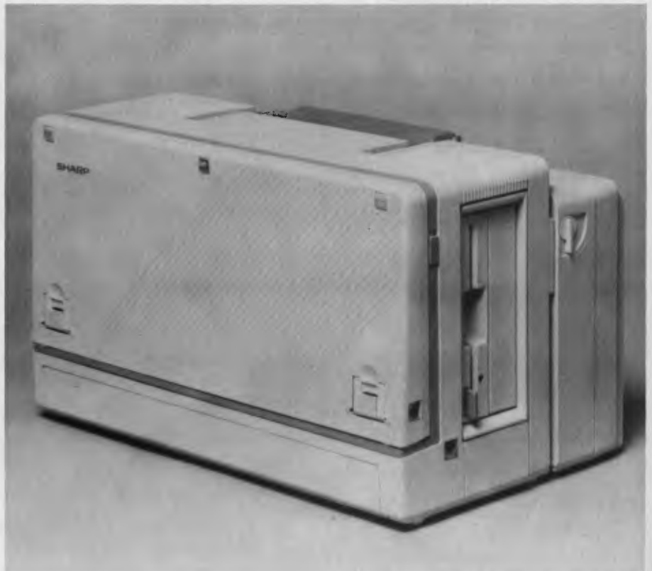
Figure 6. That nice wide handle for carrying the Sharp PC-7000 Series is a necessity: with the printer attached the unit weighs almost 14 kg (30 lb) — but the convenience of having a printer more than makes up for the weight (and bulk).
