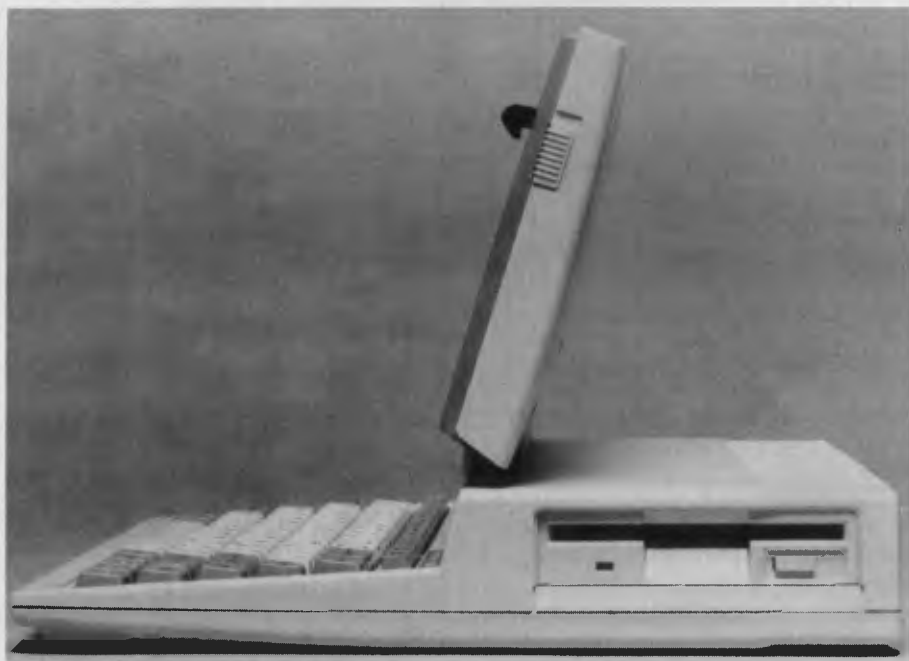
Figure 1. The Toshiba T1000 is light, neat and compact: it only weighs 2.9 kg (that's about 6.4 lb) and measures 31 cm wide, 5 high, and 28 deep (roughly 12 x 2 x 11 inches).
