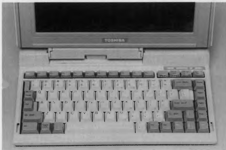
Figure 3. The Toshiba comes standard with an 84-key keyboard, but there will be a 101-key option shortly. There's an Fn key that turns the right side of the QWERTY keys into a keypad.
