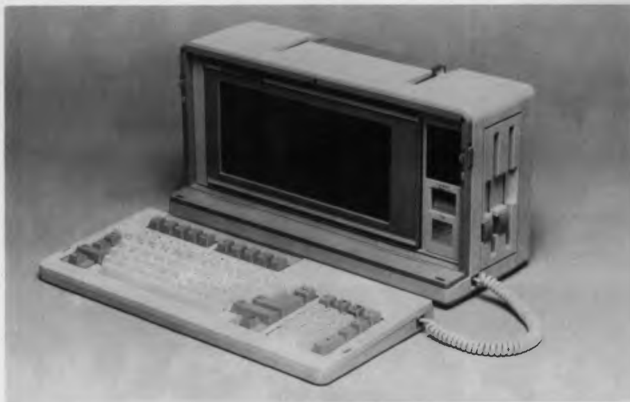
Figure 4. Sharp's PC-7000A comes with 320 kilobytes of RAM, expandable on the main board up to 704 Kbyte. It has an 80C86-2 processor with a clock speed of 7.37 MHz.
